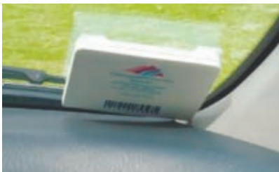
▲ Fig. 2 An RFID tag used for electronic toll collection (source: www.wikipedia.com ).
